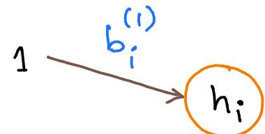
$$h_1 = \sigma(w_{11}^{(1)}x_1 + w_{12}^{(1)}x_2 + \dots + w_{1p}^{(1)}x_p + b_1^{(1)})$$
