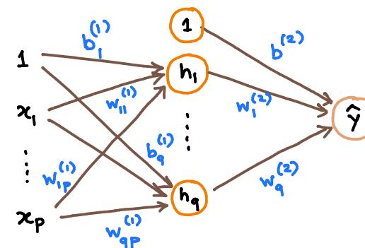
$$\begin{array}{c} \text{Column vector} \\ \underline{h} \\ q \times 1 \end{array} = \sigma \left( \underbrace{\underline{w}^{(1)} \underline{x}}_{q \times 1} + \underline{b}^{(1)} \right)$$
