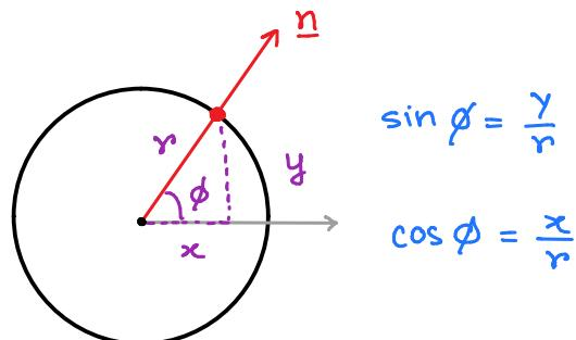
$$[\underline{n}]_{(x,y,z)} = \begin{bmatrix} \cos \phi \\ \sin \phi \\ 0 \end{bmatrix} = \begin{bmatrix} x/r \\ y/r \\ 0 \end{bmatrix}$$
