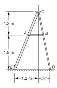
2. Estimate the force in link AB when the weight of the boat supported by the davit is 7 kN.
