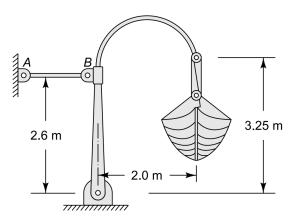
3. A spot weld which holds the bracket to the plate at point A, as shown in the figure below, can withstand a maximum bending in the plane of the plate of 100 Nm. Determine the allowable maximum load W.
