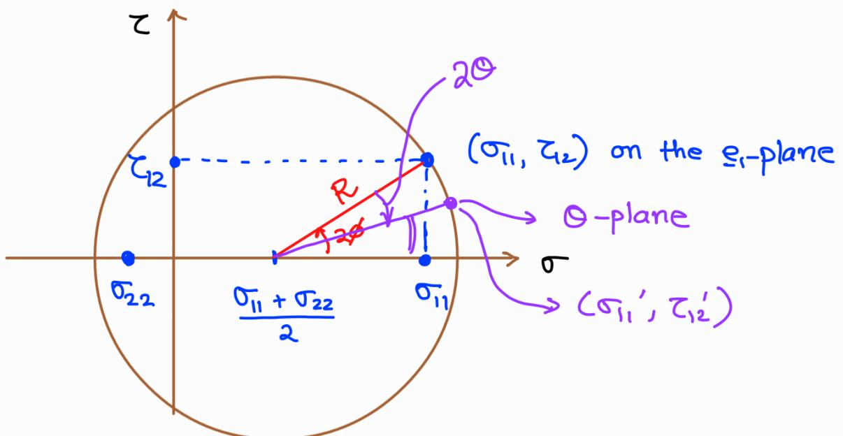
The above circle is called the 2D Mohr's circle. It can be used to find the 2D state of stress on any plane oriented at an angle  $\Theta$
