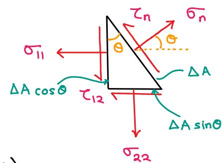
Solving the above equation, we obtain the orientation  $\Theta = \Theta_n$  of the planes of maximum and minimum normal stress
