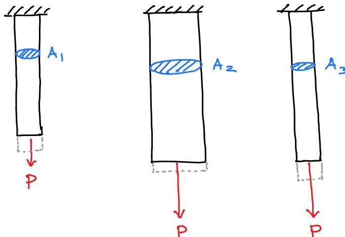
For each bar, the load is gradually increased from zero and, at several values of the load, a measurement is made of elongation ' $\delta$ '
