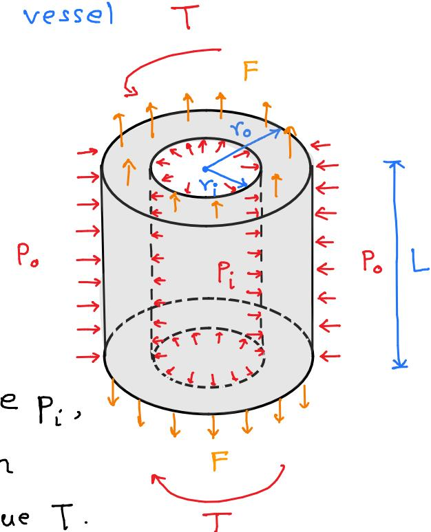
For example, for the case of a submersible hull like that of Oceangate, the important load is the outer pressure  $p_o$ .
