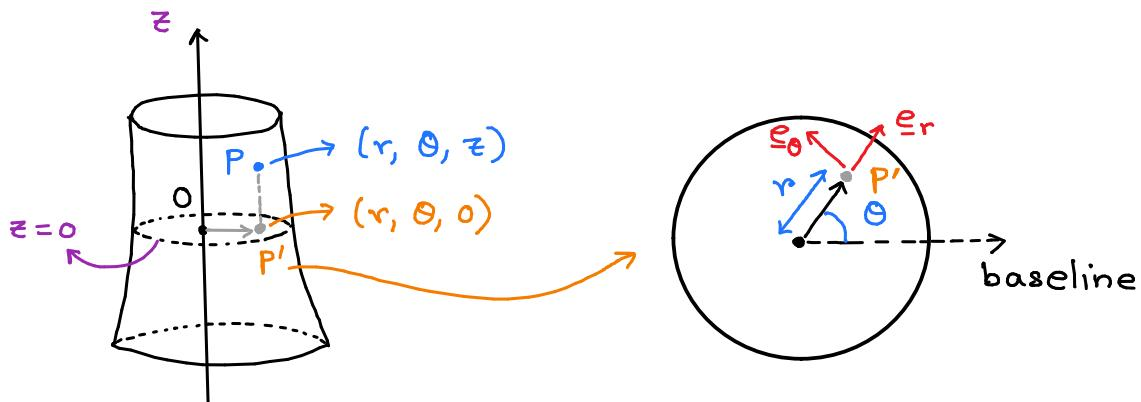
A generalized cylinder with its axis coinciding with  $z$ -axis
