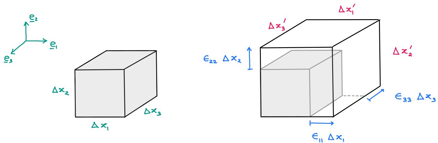
$$\left. \begin{aligned} \Delta x'_1 &= \Delta x_1 + \epsilon_{11} \Delta x_1 \\ \Delta x'_2 &= \Delta x_2 + \epsilon_{22} \Delta x_2 \\ \Delta x'_3 &= \Delta x_3 + \epsilon_{33} \Delta x_3 \end{aligned} \right\} \text{for small strains}$$
