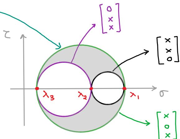
These three circles correspond to very specific normal directions i.e., they have one of their components zero. If we now plot  $(\sigma, \tau)$  for all planes with arbitrary normal directions, we will get the shaded region. This  $\sigma$ - $\tau$  plot is called the Mohr's stress plane or 3D Mohr's circle
