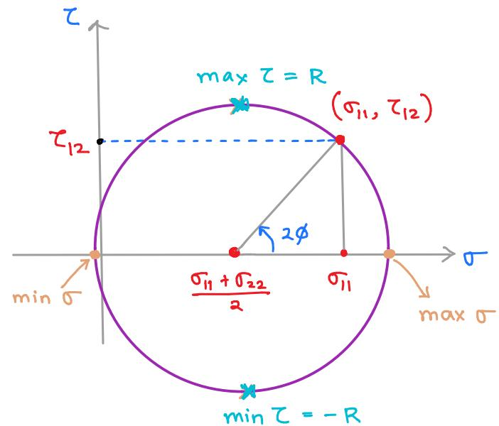
Also, note that the normal stress on the planes having maximum shear stress (topmost and bottommost points of the circle) was the  $\sigma$  corresponding to the center of the circle i.e.  $\frac{\sigma_{11} + \sigma_{22}}{2}$  or  $\frac{\lambda_1 + \lambda_2}{2}$
