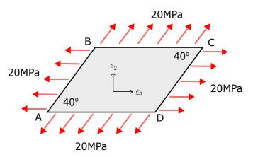
If the state of stress is uniform (i.e. it does not vary from point to point) throughout the plate, determine
