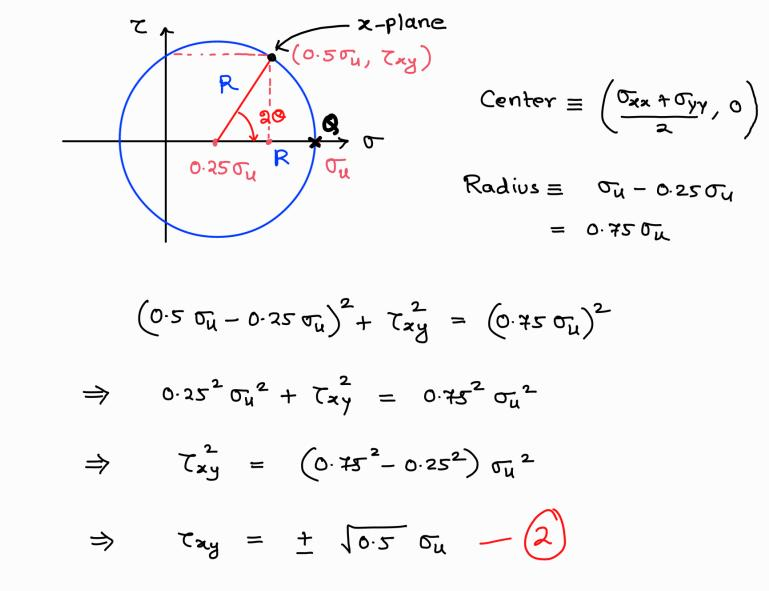
Since the torque acting on the right end of the piece of chalk is counterclockwise, the shear stress Txy acts down on the tree face of plane element and is therefore negative
