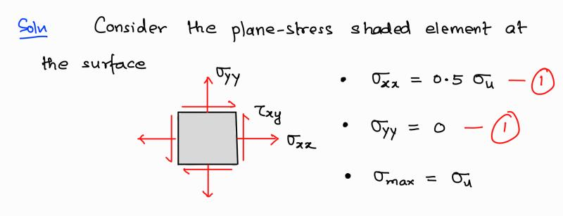
· Fracture plane orientation to be determined
