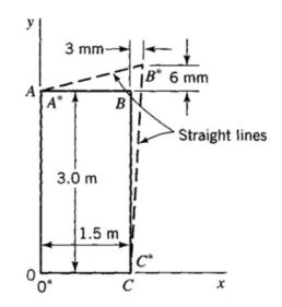
The deformed configuration of the rectangular panel is shown in dotted lines.
