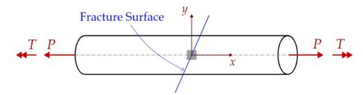
Assuming that fracture takes place when the maximum principal stress reaches the ultimate threshold strength, determine the magnitude of the torsional shear stress produced by torque T at fracture and determine the orientation of the fracture plane at the surface of the chalk with respect to the x-axis.
