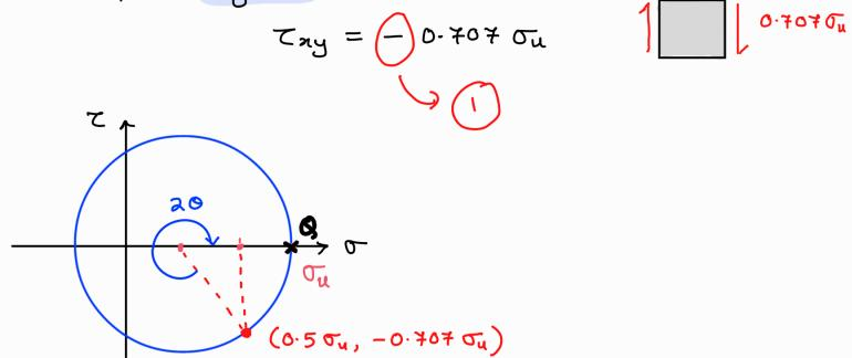
The point Q representing the max normal stress is located by rotating clockwise through 20 from ze-plane Therefore, the plane of max normal stress is physically oriented at an ongle of Q counterclockwise from z-plane normal.
