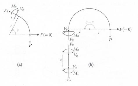
Next, we find the sectional forces and moments at an arbitrary cross-section. We take two cross-sections, one at an angle  $\theta$  from A (see subfigure (a)) and another at a distance x (see subfigure (b)).
