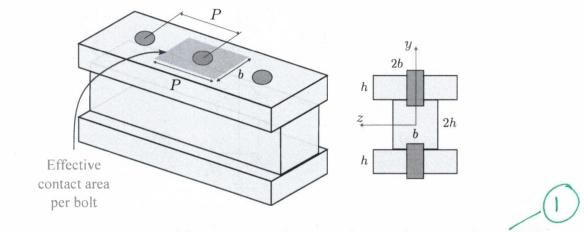
The effective area covered by each bolt has a length equal to the spacing between bolts. The total shearing force between the two planks must be resisted by the bolts.
