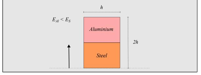
**Solution**: Composite beams are constructed from more than one material to increase their strength. In class, you have only seen beams made up of just one material. In general, the neutral axis of a composite beam will not lie at the geometric centroid of the cross-section.
