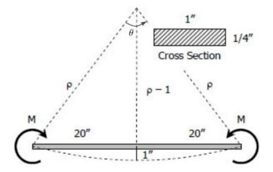
Note that the deflection of the beam is very small compared to its length. Therefore, in the above picture, we have drawn the ends of the deformed beam to coincide with the ends of the undeformed beam. In reality, the deformed beam and the undeformed beam will be of the same length due to pure bending deformation. However, with the deformed beam being curved, its two ends will be slightly inward compared to the undeformed beam. Neglecting this mismatch, we can write based on geometry that
