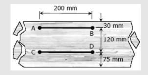
**Solution**: The picture above is that of the section of the beam along its length. The shape of the cross-section is not mentioned here. Accordingly, we can not assume that the neutral axis lies at the center. Let it lie at a distance a below the longitudinal fiber AB (see the figure below).
