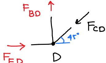
$$\begin{aligned} +\uparrow \sum F_y = 0 \\ \Rightarrow -F_{CD} \sin 45^\circ + F_{BD} = 0 \\ \Rightarrow F_{BD} = w \end{aligned} \quad \left| \begin{array}{l} +\rightarrow \sum F_x = 0 \\ \Rightarrow F_{ED} - F_{CD} \cos 45^\circ = 0 \\ \Rightarrow F_{ED} = w \end{array} \right.$$
