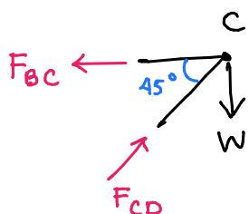
$$\begin{aligned} +\uparrow \sum F_y = 0 \\ \Rightarrow F_{CD} \cos 45^\circ - w = 0 \\ \Rightarrow F_{CD} = \sqrt{2}w \end{aligned} \quad \left| \begin{array}{l} +\rightarrow \sum F_x = 0 \\ \Rightarrow -F_{BC} + F_{CD} \sin 45^\circ = 0 \\ \Rightarrow F_{BC} = w \end{array} \right.$$
