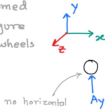
no horizontal reaction due to no brakes and castor
