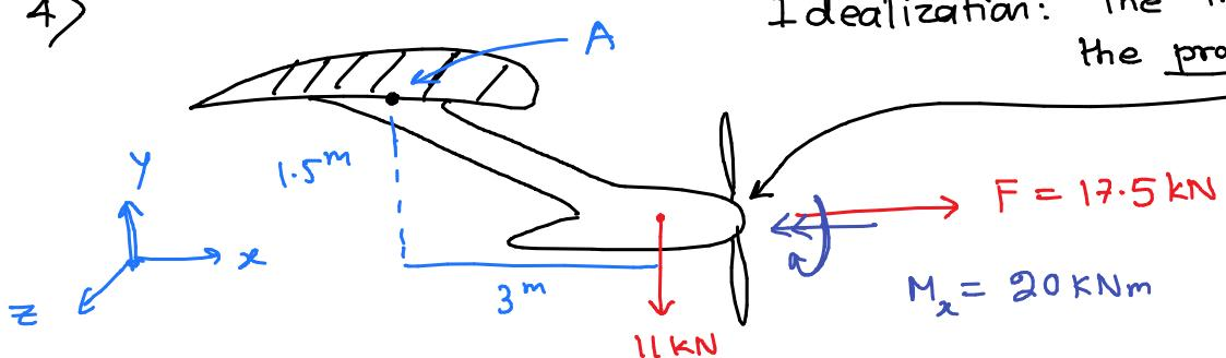
Idealization: The thrust acts through the propeller hub
