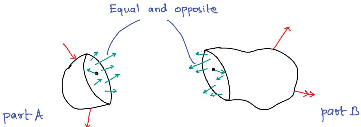
After cutting the body, if you look at the **part A** of the body, it is brought under equilibrium by a distribution of internal forces. The distribution of internal forces on **part B** must be equal & opposite according to Newton's 3rd law
