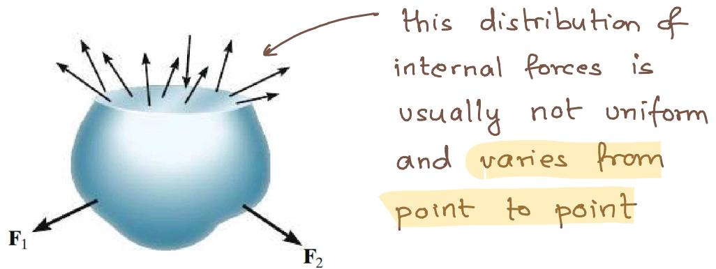
Obtaining the distribution of internal resistance in a deformable body is very important in solid mechanics
