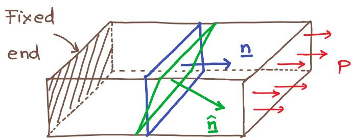
Uniform load  $P$  applied to a bar fixed at one end
