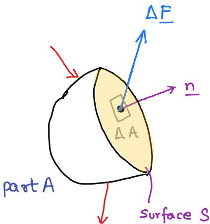
Since traction is defined as force per unit area, total surface force can be obtained from integration
