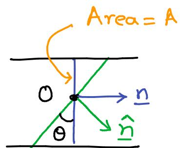
$$\text{Traction on } \begin{array}{c} \text{---} \\ | \\ \text{---} \end{array} \xrightarrow{\text{---}} \underline{\hat{n}} = \frac{P}{(A/\cos\theta)}$$
