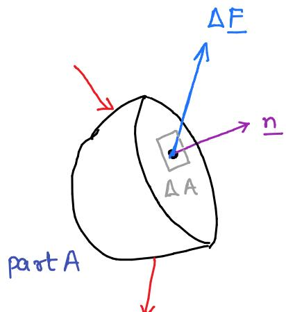
Traction vector (also called stress vector) acting at point P on a plane with unit normal  $\underline{n}$  is defined
