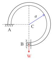
3. Determine the support reaction for the propped cantilever.
