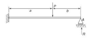
4. For the structure shown, what is the vertical deflection at end A? Also, determine the ratio of L to r if the horizontal and vertical deflections of the loaded end A are equal. P is the only force acting
