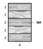
The allowable shear stress in the glue is 90 psi, the allowable shear stress in the wood is 120 psi, and the allowable flexural stress in the wood is 1200 psi. Determine the maximum uniformly distributed load that can be carried by a simply supported beam on a 6ft simple span.
