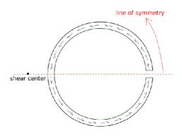
5. Think of a beam having thin and open cross-section. The shape of the cross-section is shown in the figure. Suppose the beam is subjected to a transverse load at one of its end such that the force applied is along 'Y' axis.
