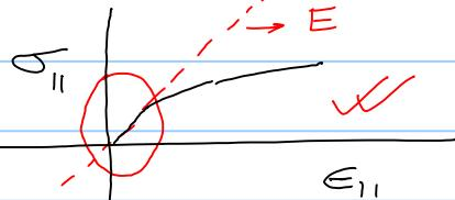
$$\boxed{\text{Graph for uniaxial tensile test}} \quad \frac{d\sigma_{11}}{d\epsilon_{11}} \Big|_{\epsilon_{11}=0} = E$$
