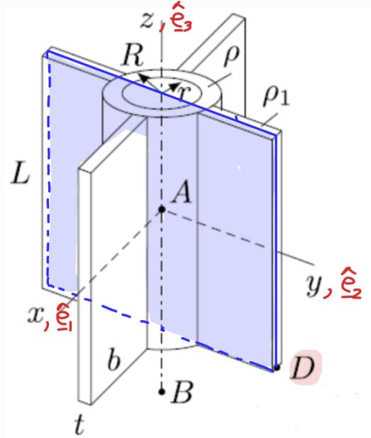
$$\begin{bmatrix} \underline{\underline{I}}^D \\ \left( \begin{array}{c} \hat{e}_1 \\ \hat{e}_2 \\ \hat{e}_3 \end{array} \right) \end{bmatrix} = \begin{bmatrix} I_{xx}^D & 0 & 0 \\ 0 & I_{yy}^D & I_{yz}^D \\ 0 & I_{zy}^D & I_{zz}^D \end{bmatrix}$$
