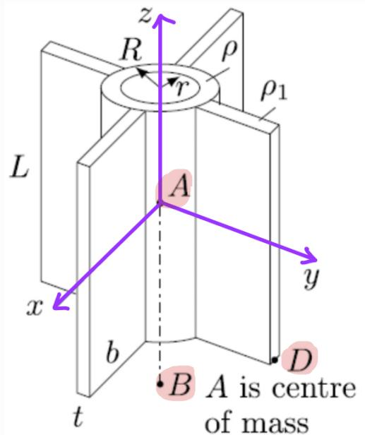
Find principal axes of the composite RB at point A, B, and D.
