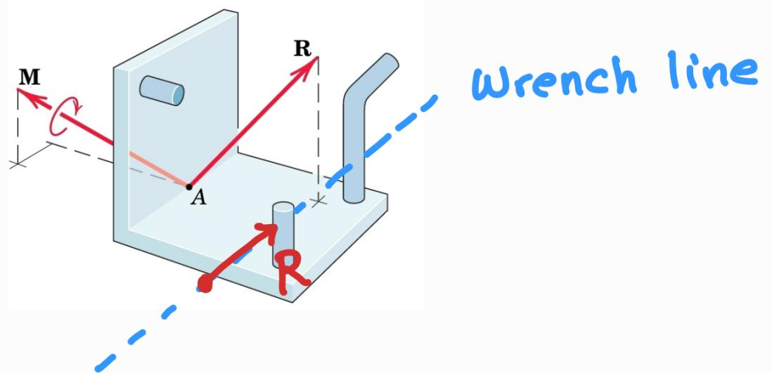
3> Find the equivalent force system at point A and the wrench location.
