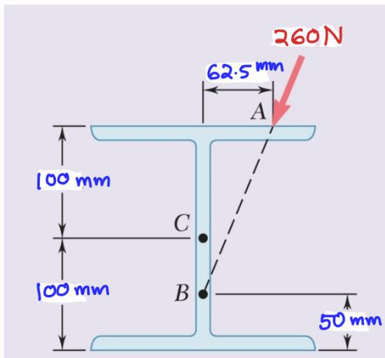
A 260 N force is applied at A to the rolled-steel section.
