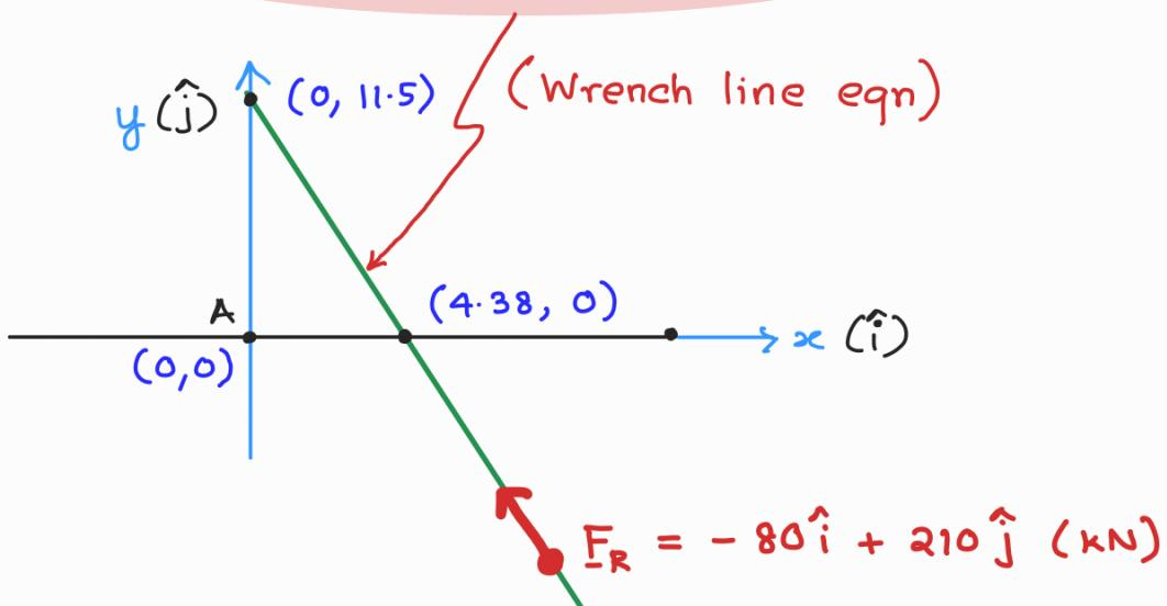
You can place  $\underline{F}_R$  at any point on the wrench line and you will still get the same resultant couple  $\underline{C}_{RA}^{\perp}$  at A.
