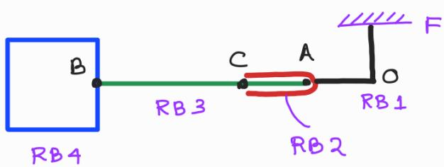
\* RB<sub>3</sub> (rod BC) is extending outwards wrt RB<sub>2</sub>
