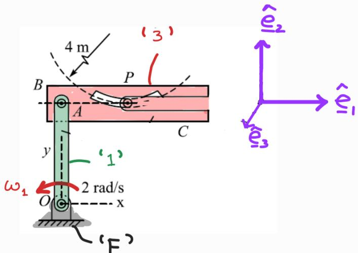
$\underline{v}_{A/F}$  can be obtained by treating I.F.  $\equiv '1'$  and I.P.  $\equiv 'O'$
