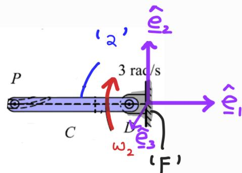
$$\underline{r}_{PD} = \underline{r}_P - \underline{r}_D = -2 \hat{\underline{e}}_1 \text{ (m)}$$
