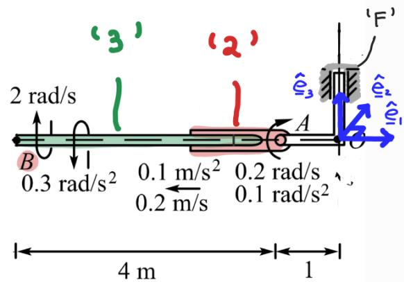
$$\underline{x}_{BA} = \text{Position vector from } A \text{ to } B = \underline{x}_{B/0} - \underline{x}_{A/0} = -4 \hat{\underline{e}}_1 \text{ (m)}$$
