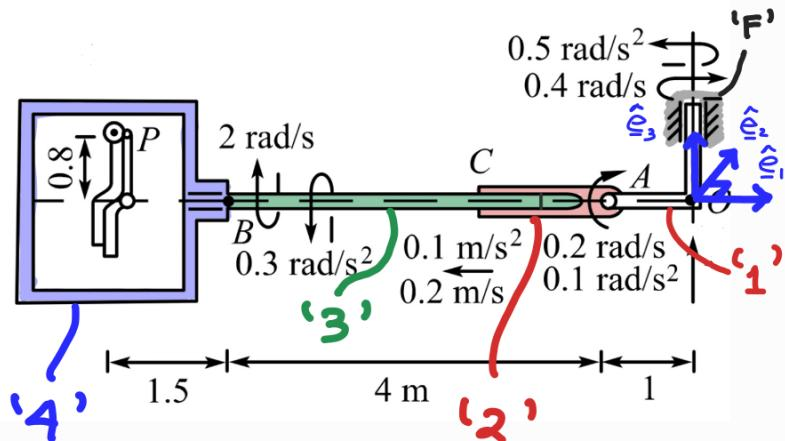
Velocity and acc of a pt B on RB ' $3$ ' w.r.t. RB ' $2$ '
