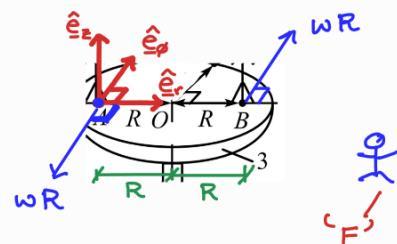
$$\underline{v}_{BA}|_m = \underline{v}_B|m - \underline{v}_A|m = \underline{\Omega}$$
