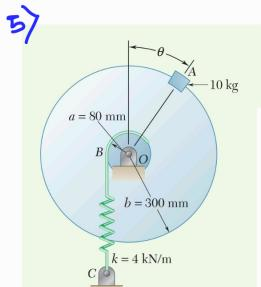
A 10-kg block is attached to the rim of a 300-mm-radius disk as shown. Knowing that spring BC is unstretched when  $\theta = 0$ , determine the position or positions of equilibrium, using PVW.
