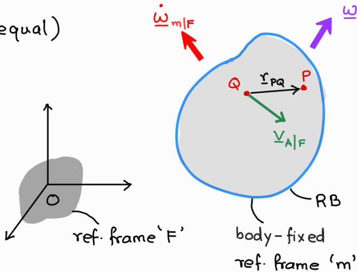
Since the points of the RB are fixed wrt body-fixed ref frame 'm', their motion wrt frame 'F' can be obtained by composition formulae:
