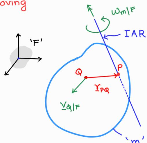
It can be shown that non-zero velocity vectors (e.g.  $v_{Q/F}$ ) of all other points of the RB must be  $\perp$  to  $\omega_{m/F}$ , if there exists an IAR through (say) point P of the RB.
