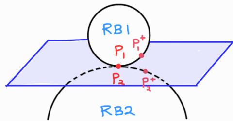
Along the tangential plane of contact, the acceleration components of  $P_1$  and  $P_2$  are the same at time instant ' $t$ '
