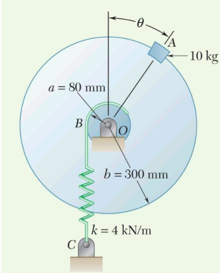
A 10-kg block is attached to the rim of a 300-mm-radius disk as shown. Knowing that spring  $BC$  is unstretched when  $\theta = 0$ , determine the position or positions of equilibrium, using PVW.
