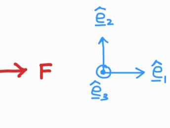
The uniaxial force required to stretch (or compress) the spring is given by  $F = kx \hat{e}_1$ , which is a linear force of the type  $F_L(x) = \alpha x$
