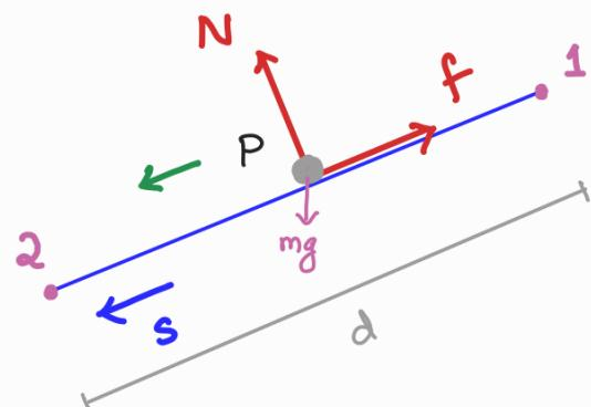
2) the normal force remains constant, both in magnitude and direction, along the path 's' i.e.  $N(s) = N$
