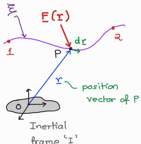
$$W = \int_{\xi} \underline{F}(\underline{r}) \cdot d\underline{r} = \int_{\underline{r}_1}^{\underline{r}_2} \underline{F}(\underline{r}) \cdot d\underline{r}$$
