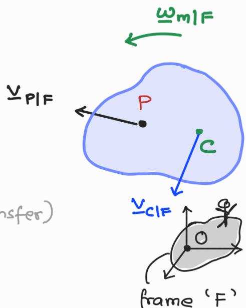
$$v_{P/F} = v_{C/F} + \omega_{m/F} \times r_{PC} \quad (\text{vel. transfer})$$
