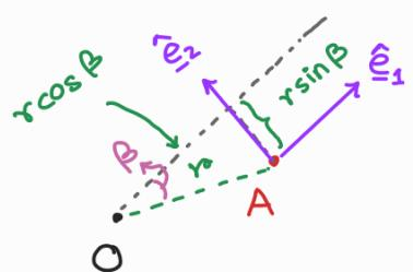
$$\begin{aligned}\text{Angular velocity of rod, } \underline{\omega}_{2|F} &= \underline{\omega}_{1|F} + \underline{\omega}_{2|1} \\ &= (\omega + \dot{\beta}) \underline{e}_3\end{aligned}$$
