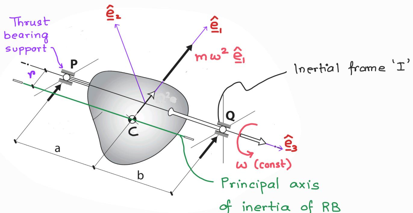
Rotor imbalance is caused due to unsymmetric mass dist.
