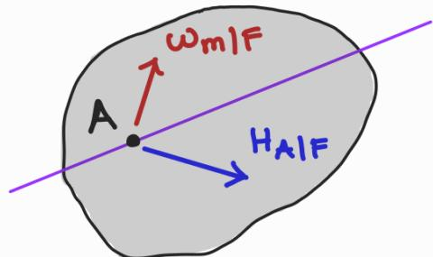
However, for each point A, there are some directions/axes for which the two vectors  $\underline{\omega}_{mif}$  and  $\underline{H}_A$  are parallel. These directions are called principal directions and the axes along these directions are called principal axes of inertia at that point.
