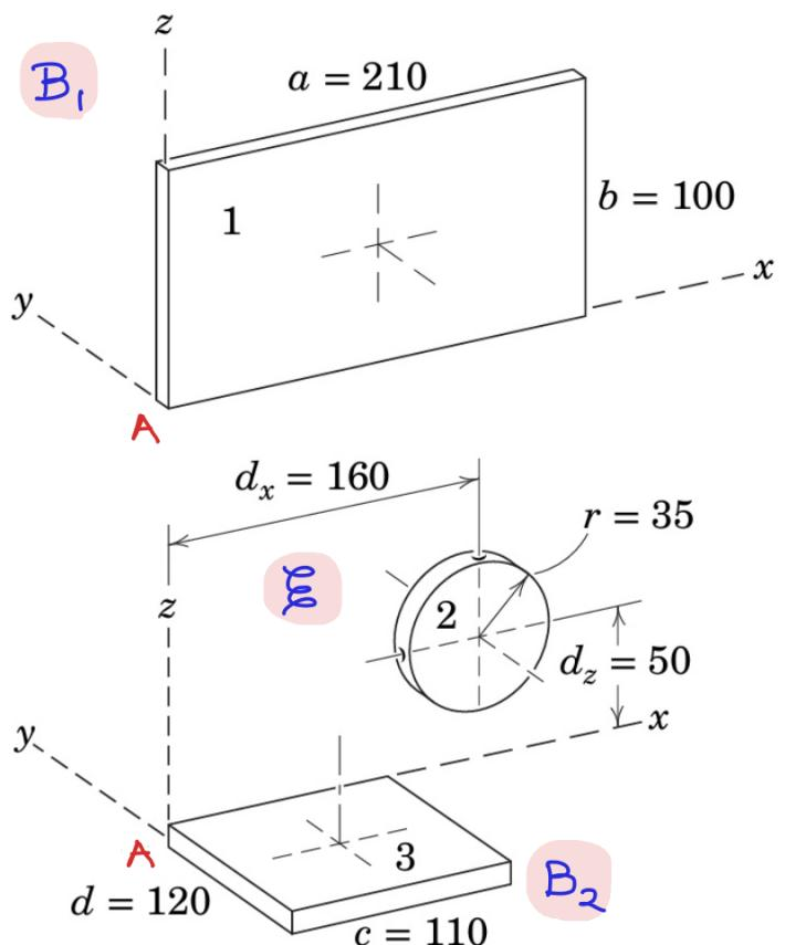
$$[\underline{\underline{I}}^A](B_1) = \begin{bmatrix} \frac{1}{3}mb^2 & 0 & -\frac{mab}{4} \\ 0 & \frac{1}{3}m(a^2+b^2) & 0 \\ -\frac{mab}{4} & 0 & \frac{1}{3}ma^2 \end{bmatrix}$$
