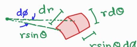
$$\begin{aligned} I_{33}^c &= \int (x^2 + y^2) dm \\ &= \int (rsin\theta)^2 \rho \, rd\theta \, rsin\theta \, d\phi \end{aligned}$$
