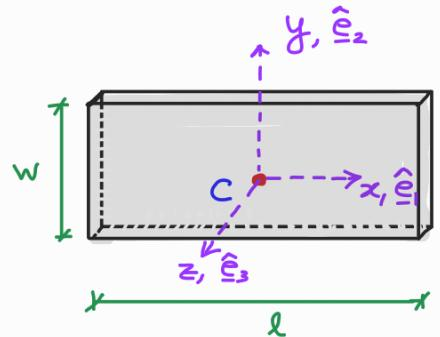
$$[\underline{\underline{I}}^c] = \begin{bmatrix} \frac{m\omega^2}{12} & 0 & 0 \\ 0 & \frac{m\ell^2}{12} & 0 \\ 0 & 0 & \frac{m(\ell^2 + w^2)}{12} \end{bmatrix}$$
