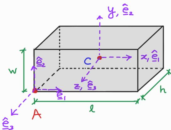
$$I_{11}^A = I_{11}^C + m \underbrace{(x_{c_2}^2 + x_{c_3}^2)}_{d_1^2}$$
