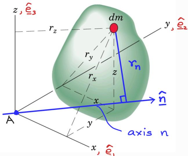
These integrals are always positive, whereas the products of inertia  $I_{12}^A = \int xy dm$ ,  $I_{13}^A = \int xz dm$ , and  $I_{23}^A = \int yz dm$  may be positive, negative, or zero.
