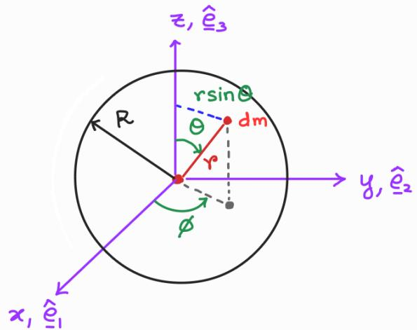
and  $I_{11}^c = I_{22}^c = I_{33}^c$  (since the sphere is symmetric about any axis passing through c)
