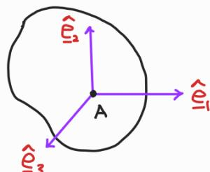
$$\left[ \underline{\underline{I}}^A \right] = \begin{bmatrix} I_{11}^A & I_{12}^A & I_{13}^A \\ I_{21}^A & I_{22}^A & I_{23}^A \\ I_{31}^A & I_{32}^A & I_{33}^A \end{bmatrix}$$
