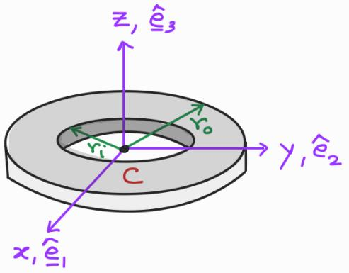
$$[\underline{\underline{I}}^c] = \begin{bmatrix} \frac{m(r_o^2 + r_i^2)}{4} & 0 & 0 \\ 0 & \frac{m(r_o^2 + r_i^2)}{4} & 0 \\ 0 & 0 & \frac{m(r_o^2 + r_i^2)}{2} \end{bmatrix}$$
