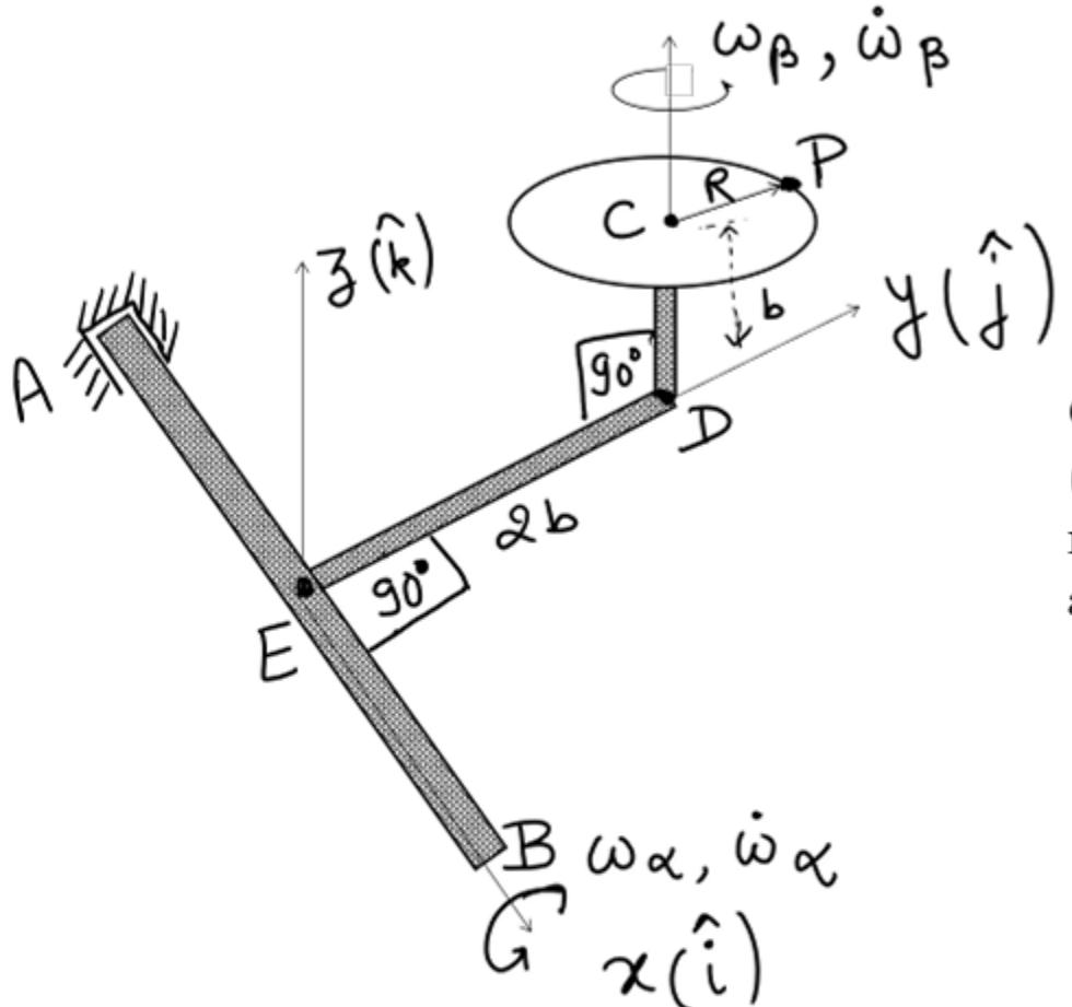
**Q1) [7 points]** Rods AEB and EDC are welded together (rigid body 1). A is a ball-and-socket joint. This assembly rotates relative to the ground frame with angular velocity and angular acceleration  $\omega_\alpha$  and  $\dot{\omega}_\alpha$
